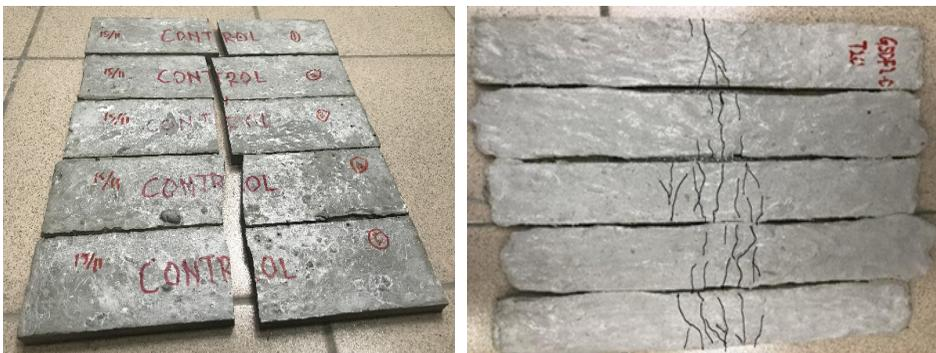
Figure 5. Failure modes under three-point bending test
